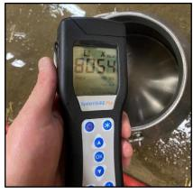
ATP Monitor pictured above is used to determine how clean a surface or feeding equipment is.
